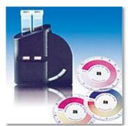
system. The two cells are filled with the water sample and one is placed directly into the left-hand compartment of the comparator, where it acts as compensation (blank) for coloured, or cloudy samples.
